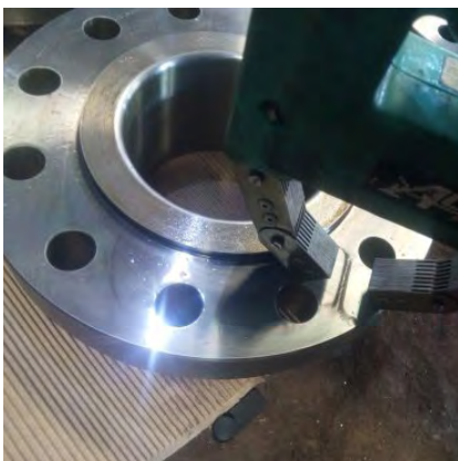
MAGNETIC PARTICLE INSPECTION
