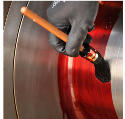
DYE PENETRANT TESTING
